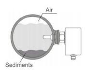
For horizontal mount, avoid probe touching air or sediments. At least half of probe should be immersed in the medium.
