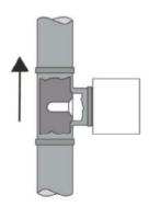
For vertical mount, make sure medium flows upward. At least half of probe should be immersed into medium.
