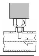
When mounting, the mark "X" should always face flow direction to have the best performance.
