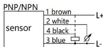
1 switching output + 1 analog output
